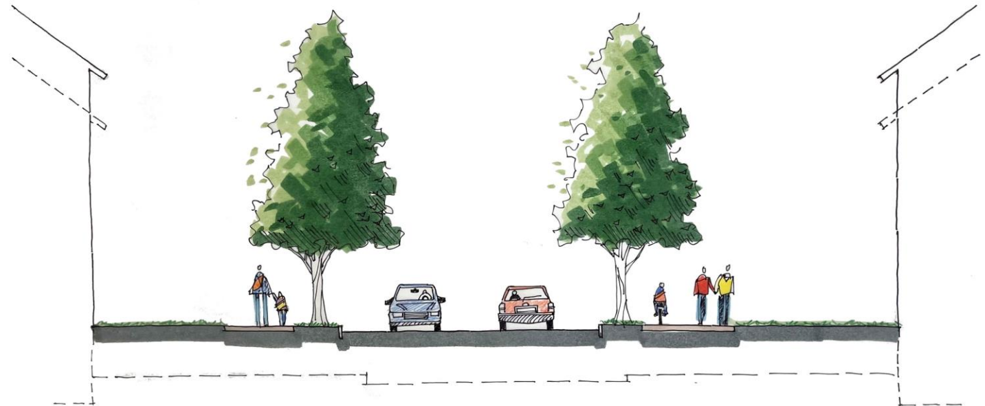
Two cross-sections demonstrating road elevation options within the Resilient Corridor with accompanying structure elevations. Streetscape additions could include an off-street shared-use path, green infrastructure, and building elevations tying into the raised road.
